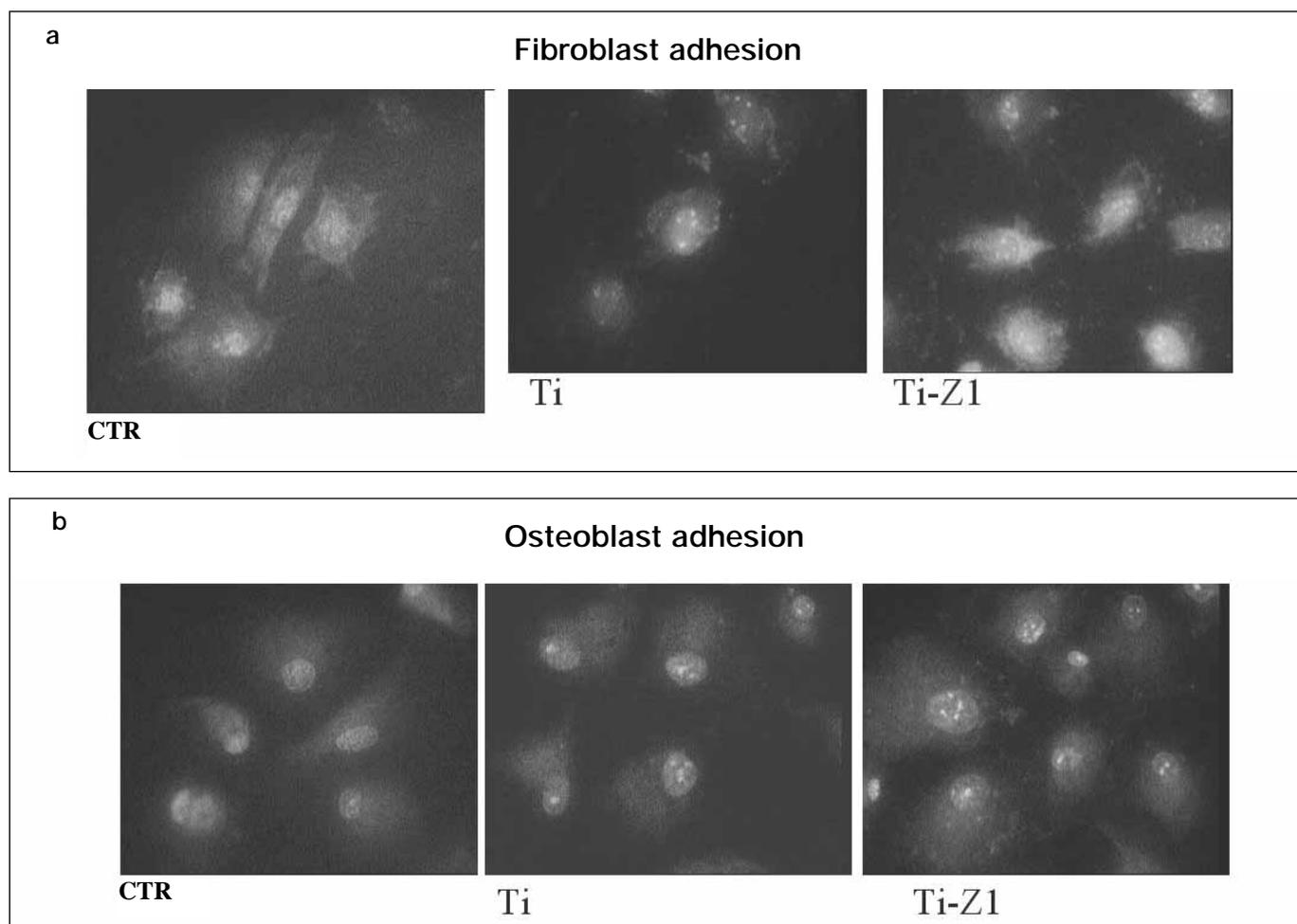
**Fig. 4** - Morphology of fibroblasts (a) and osteoblast-like cells (b) adhesion on cell culture dish, titanium and zirconia coated titanium. Materials were incubated for 6 hr with fibroblasts and human osteoblast-like cells. Samples were examined by fluorescence microscopy at 250× magnification.
