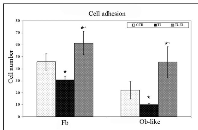
Fig. 2 - Fibroblasts and osteoblast-like cells quantification at 6 hr cell incubation (adhesion test) on titanium (Ti), zirconia coated titanium (Ti-Z1) and on control Thermanox® slide (CTR). Cell number was the mean of 20 measurements in three experiments (n=60) and was referred to a surface area of 0.1715 mm². \* p < 0.05 with respect to controls; ° p < 0.05 with respect to Ti.
